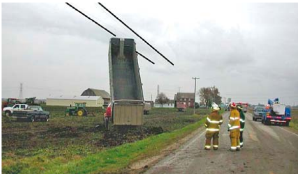
Extended trailer bed touching power lines (lines enhanced for clarity)
