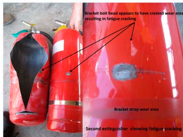
Actual Bracket Involved Arrows point to bolt location
