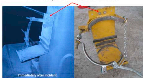
Actual Bracket Involved Arrows point to bolt location
